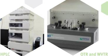
A vital device for the separation and identification of components in a mixture such as colorants, sweeteners, sugars, aflatoxin, ochratoxin
